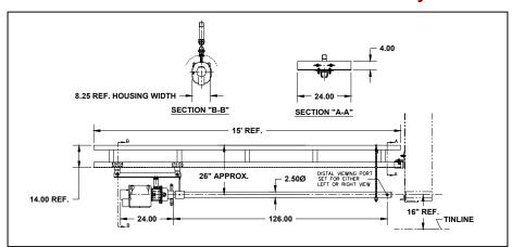
The optional monorail assembly includes a reinforced monorail track for mounting to the tin bath. The periscope is coupled to a trolley assembly by way of two mounting sleeves.
